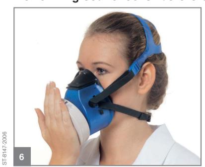
Seal the respiratory filter with your hand and breathe in until a negative pressure (suction) is generated. Hold your breath for a moment. The negative pressure should be maintained. If not, readjust the face piece and adjust the straps or use a different size of mask. Repeat test until a successful seal check is met.
