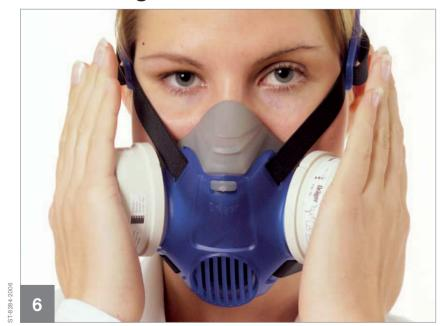
Negative pressure test: Seal both respiratory filters with your hands and breathe in until a negative pressure (suction) is generated. Hold your breath for a moment. The negative pressure should be maintained. If not readjust the face piece and adjust the straps or use a different size of mask. Repeat test until a successful seal check is met.
