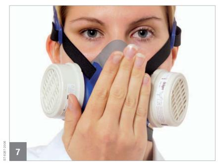
Positve pressure test: Seal the exhalation valve of half mask and exhale. The half mask will inflate slightly. If the exhaled air leaks out of the mask, readjust the face piece and adjust the straps or use a different mask size. Repeat test until a successful seal check is met.
