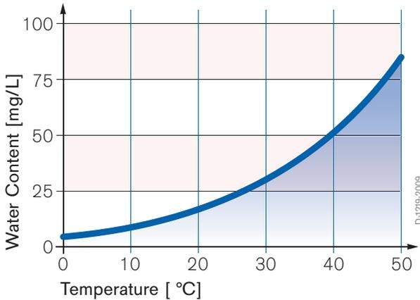
The maximum water vapor content of the air depends on temperature, i. e. the figures of relative humidity are always to be considered in reference to temperature. To convert relative humidity into absolute humidity as a function of temperature, the above diagram or the following formula can be used. Using a pocket calculator a conversion can be done:
