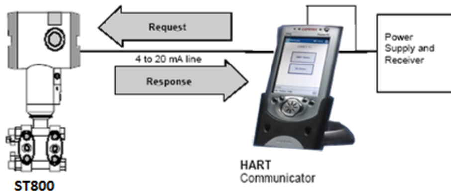
Figure 1 Typical Communication Interface
