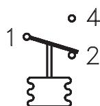
**NOTICE**, there are two different ways of working for pressure limiter: one as a pressure limiter for rising and another one as a pressure limiter for falling. For identification, there is adequate description on the bottom of housing (see below examples).
