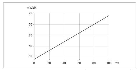
Figure 1-3: Temperature dependency of the Nernst Factor (theoretical slope of a pH sensor)
