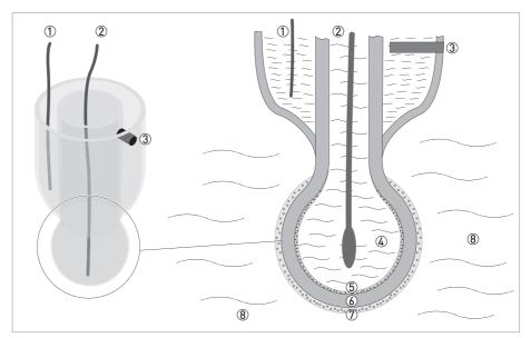
Figure 1-1: Measuring principle for pH measurement
