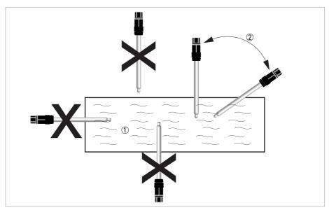
Figure 3-2: Installation requirements
