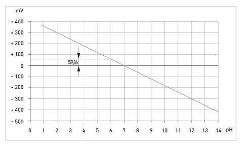
Figure 1-2: Optimal slope at  $25^{\circ}$ C /  $77^{\circ}$ F
