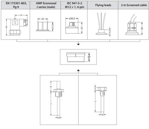
E = Extension length = 33 mm L = Insertion lengthH = 9 mm
