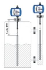
With special versions it is possible to measure the level of the interface between two immiscible liquids of different densities. The displace rod must be covered completely with liquid. The difference in density should be min. 100 g/l.
