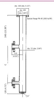
Dimension C = Distance between sockets (measuring range)
